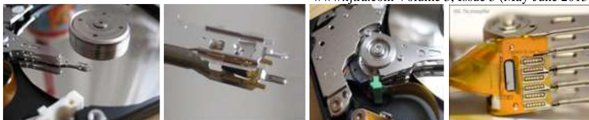
Figure 9: Read & Write Head of HDD
