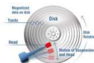
Figure 8: HDD operation motion
