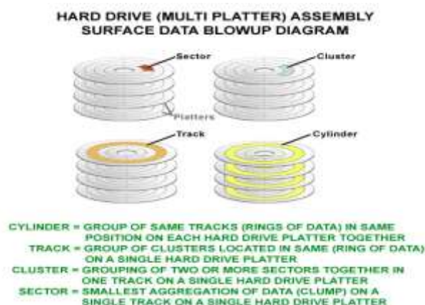
Figure 10: Multi Platter Surface of HDD
